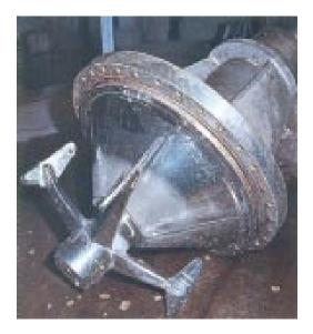
Conditions were so severe in C-stage bleaching operations at one mill that even C-276 alloy welds were suspect. As a preventive maintenance measure, 3 mm was ground off each weld and replaced with a weld deposit of C-22 alloy. This photo, taken 18 months later, shows the welds virtually unaffected. At this printing, it is still in service after 7 years.
