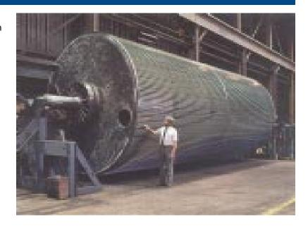
Solid rocket propellant effluents and salt air caused pitting and crevice corrosion attack of stainless steel. C-22 alloy was selected over 19 different alloys for the clamshell bellows after extensive testing. The bellows have been in service for more than 12 years.
