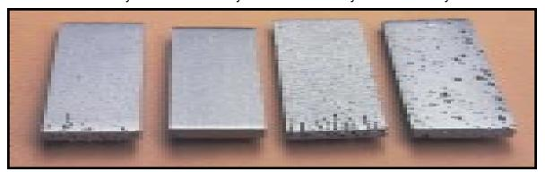
Samples were subjected to a solution of 11.5%  $\rm H_2SO_4$ , 1.2%  $\rm HCI$ , 1%  $\rm FeCl_3$  AND 1%  $\rm CuCl_2$ . Solutions for coupons 625 and C-4 were at 102°C, while C-276 and C-22 were at 125°C.
