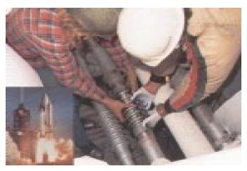
Sleeved electrogalvanizing finishing rolls made of HASTELLOY C-22 alloy are ready for placement in a steel finishing manufacturing line. C-22 alloy helps reduce defects on the rolls which is necessary to produce defect free galvanized steel for the automotive industry.
