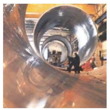
The largest fabrication of HASTELLOY® C-22® alloy known to-date is shown here being thin-sheet lined for exposure in a utility flue-gas desulfurization plant. C-22 sheet is still providing excellent service after 10 years.
