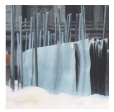
HASTELLOY<sup>®</sup> G-30<sup>®</sup> alloy has outstanding resistance to hydrofluoric/nitric acid mixtures such as employed in the pickling of stainless steel. This particular operation involves aerated, 15% HNO<sub>3</sub> and 5% HF at 140 deg. F. (60 deg. C)
