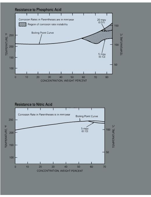
\*All test specimens were heat-treated at 2150°F (1177°C), rapid quenched and in the unwelded condition.
