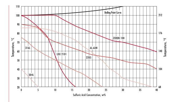
Sulfuric Acid Iso-corrosion Curves, 4 mpy Stainless Steels
