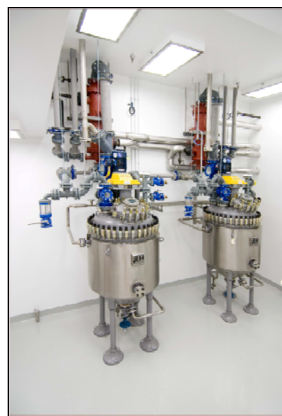
TANTALUM PHARMACEUTICAL CONDENSERS INSTALLED WITH GLASS LINED STEEL REACTORS
