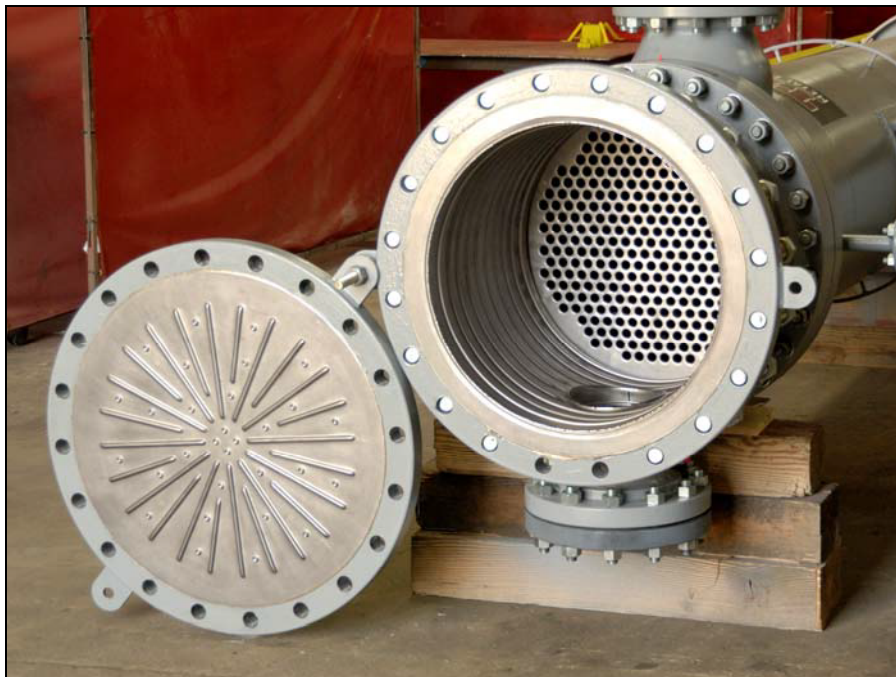
32" DIAMETER X 20 FEET LONG TANTALUM HEAT EXCHANGER
