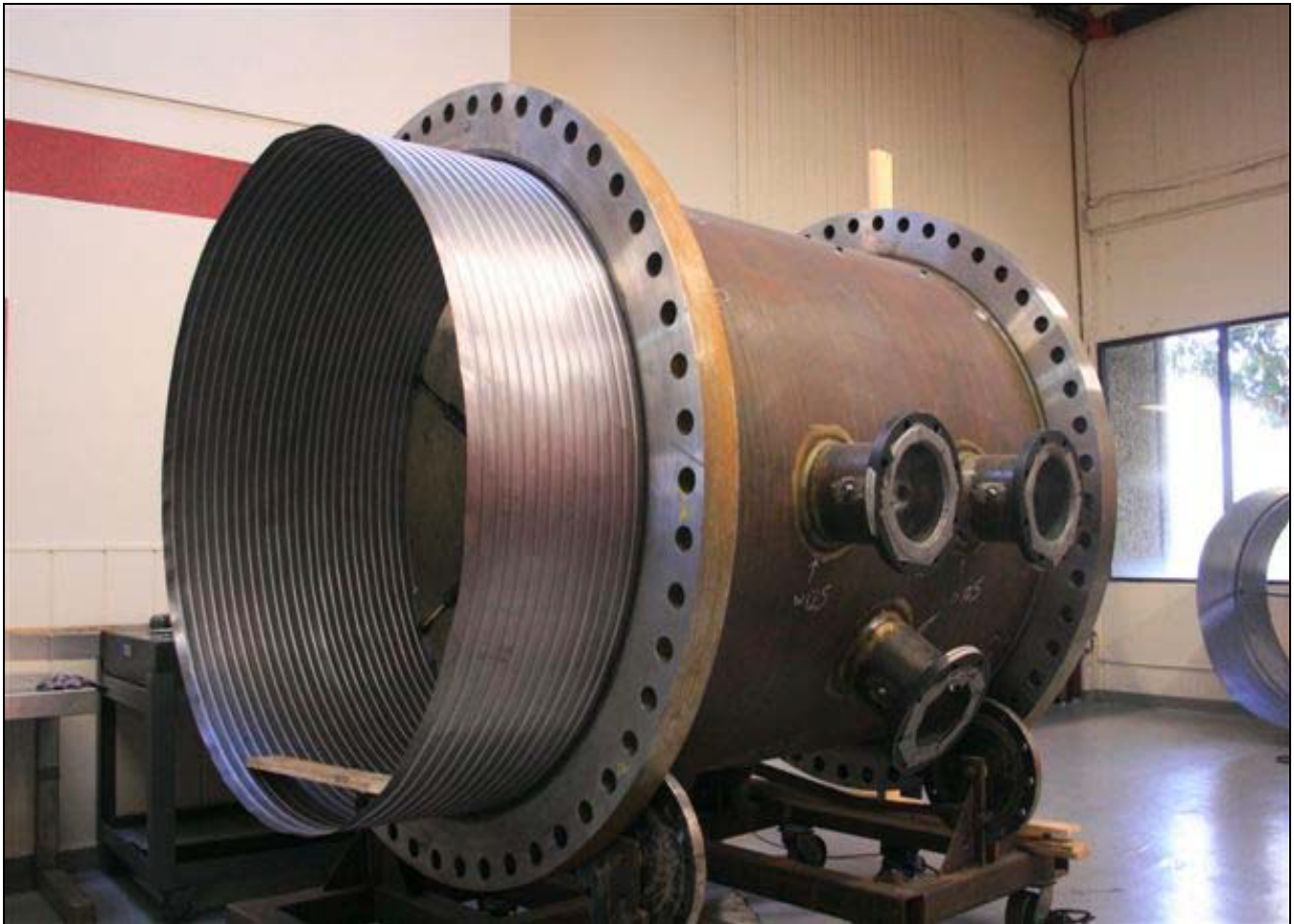
TANTALUM LINED CARBON STEEL PRESSURE VESSEL
