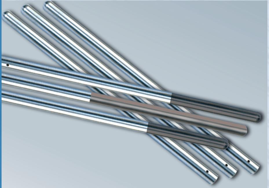
Optimum Anode Technologies' rod and custom shape anodes for cathodic protection are MMO (Mixed Metal Oxide) IrOxide™ Series coated titanium substrates. These rods and custom shape anodes consist of Iridium as the main constituent of the electrochemical catalyst, providing both excellent electrochemical catalytic activity and stability in a chlorine or oxygen evolving environment. The rods are frequently in seawater, brackish water, freshwater and coke breeze as well as other environments.
